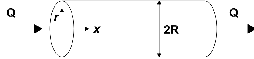
Figure 4.12: Flow through a circular tube
