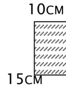
$$D = \sqrt{\frac{6 \cdot S}{B}} = \sqrt{\frac{6(335.50 \text{CM}^3)}{10 \text{CM}}} = 14.18 \text{CM} \quad S = \frac{B \cdot D^2}{6} = \frac{10(15)^2}{6} = 375 \text{CM}^3$$
