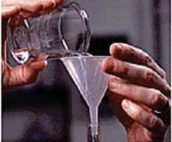
To fill a buret, close the stopcock at the bottom and use a funnel. You may need to lift up on the funnel slightly, to allow the solution to flow in freely.
