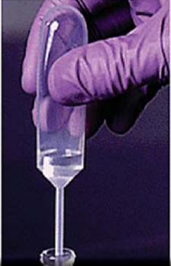
You can also fill a buret using a disposable transfer pipet. This works better than a funnel for the small, 10 mL burets. Be sure the transfer pipet is dry or conditioned with the titrant, so the concentration of solution will not be changed.
