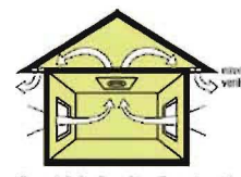
Figure 8.8: Cooling with ceiling exhaust fan
