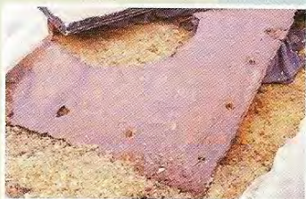
Armored deck plating recovered from the wreck of the USS Monitor lies in a packing crate on board the Kellie Chouest off Cape Hatteras Tuesday. The plate, originally 2 inches thick, was paper-thin in some areas. Rivet holes surround the edge of the iron plate.
