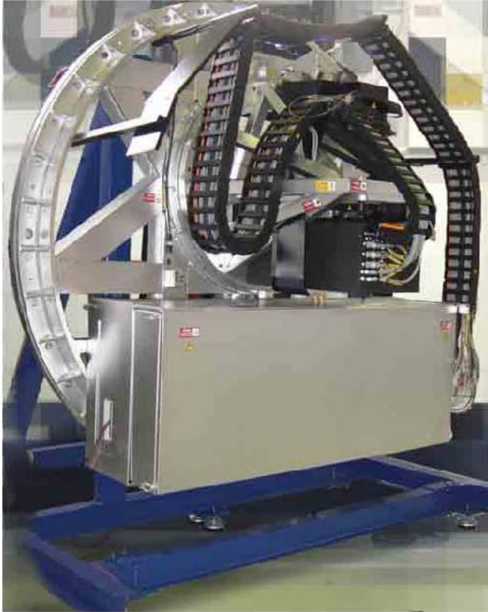
Figure 6: Electronics cabinet attached to CI structure.
