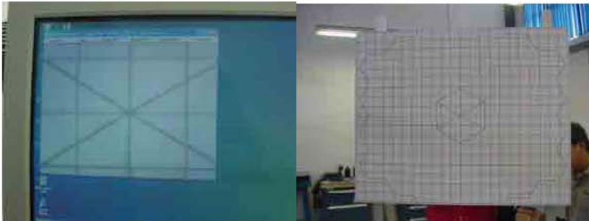
Figure 4: Collimator pupil distortion test.
