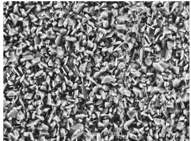
Fig. 8 SEM micrograph on surface of \text{YVO}_3 compound at 850 °C, one can observe how grain size decreases with an average around 2.87 \pm 0.10 \mu\text{m} , and at the same time the distribution is homogeneous
