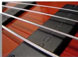
Pick Ups o pastillas electromagnéticas
