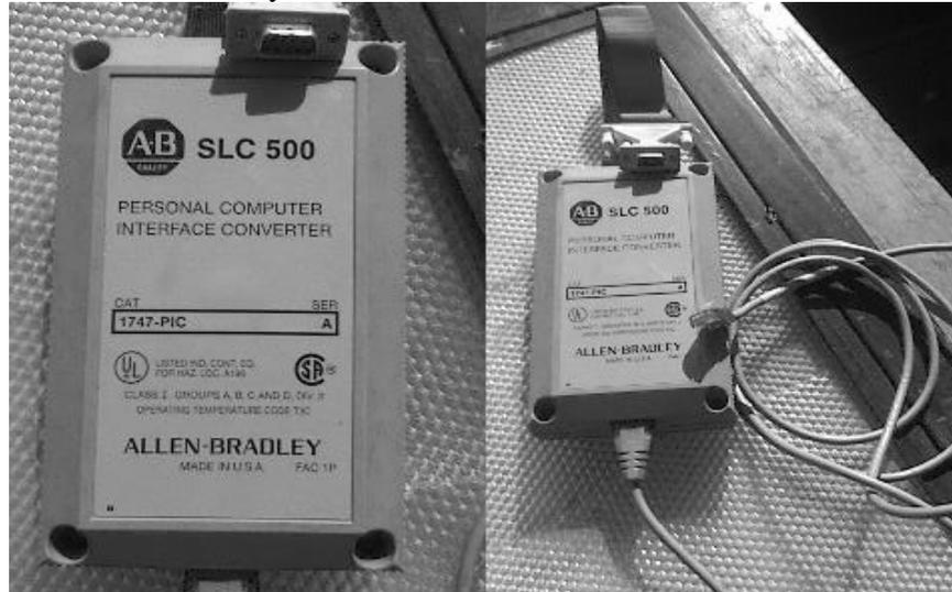
Fig. 5.29 Modem Conversor Serial-Ethernet 1747-PIC.
