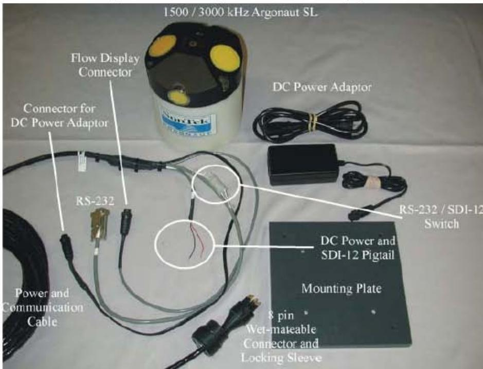
Figure 5-14. 1500 or 3000-kHz Argonaut-SL with Standard Equipment
