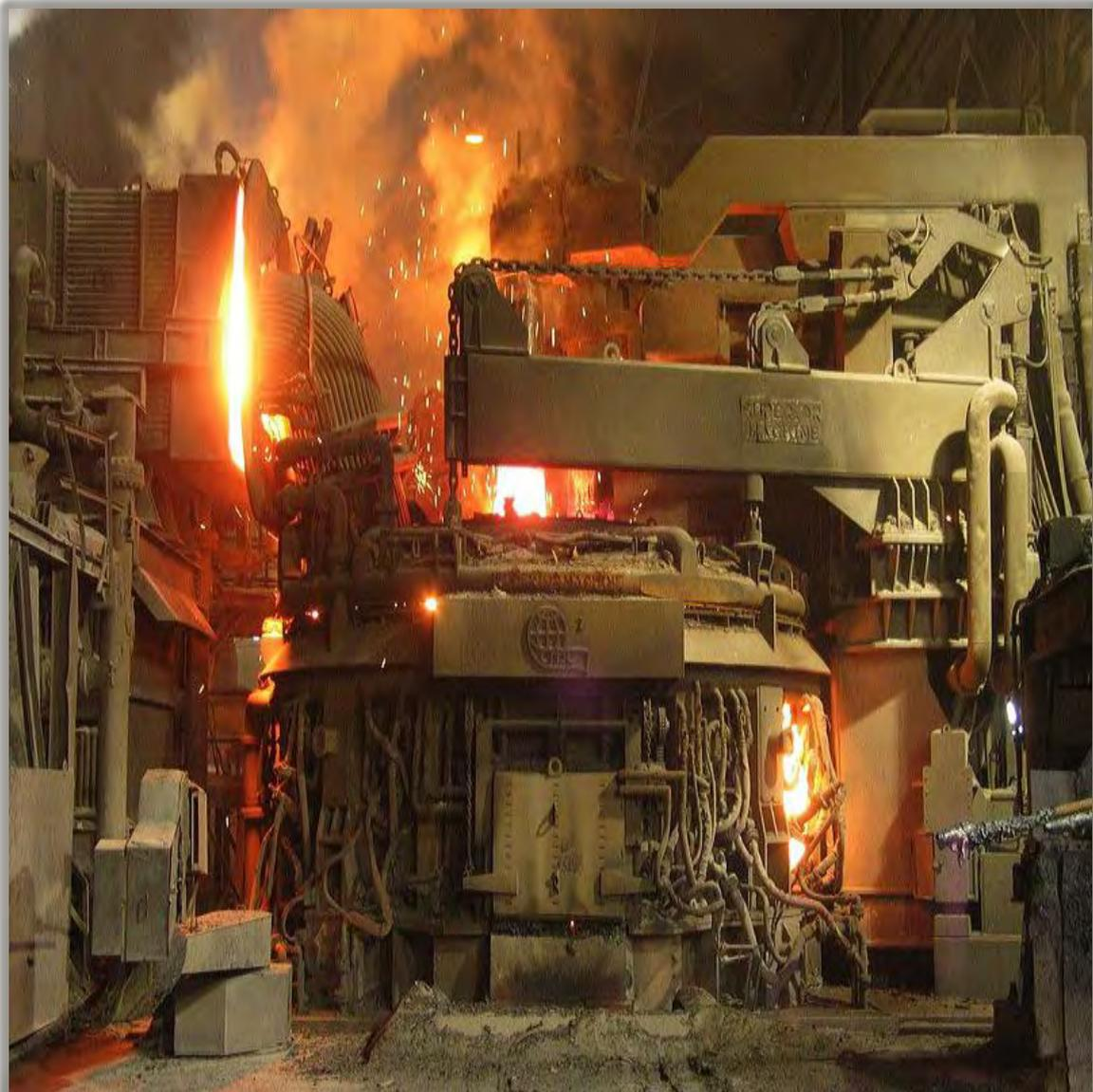
FIGURA 2.13 HORNO DE ARCO ELECTRICO
