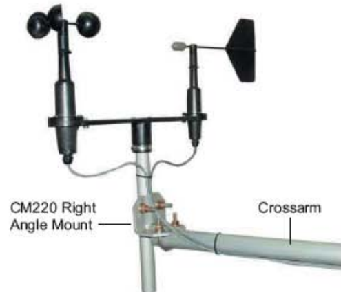
The 03001 is secured to one end of the CM206 Crossarm with the CM220 Right Angle Bracket.
