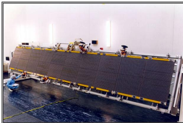
Fig. IV.6.2. Antena ASAR (Advanced Synthetic Aperture Radar).
