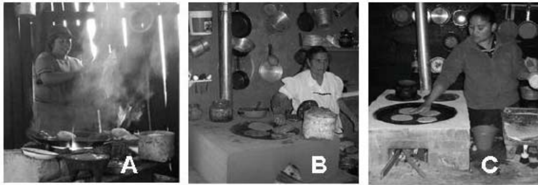
Figure 1. Traditional open fire (A), mud-cement Patsari (B), and brick Patsari (C) (Photo: M. Johnson)
