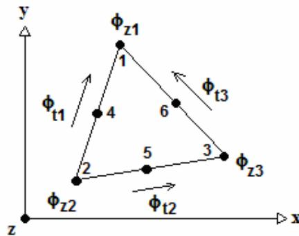
**Fig. 3.5 Elemento orilla triangular**
