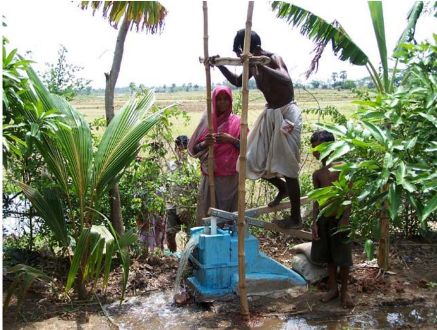
**Figura 26 Bomba de Pedal**
