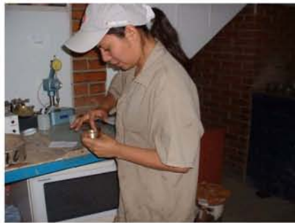
Figura 4.28 Engrasado de moldes
