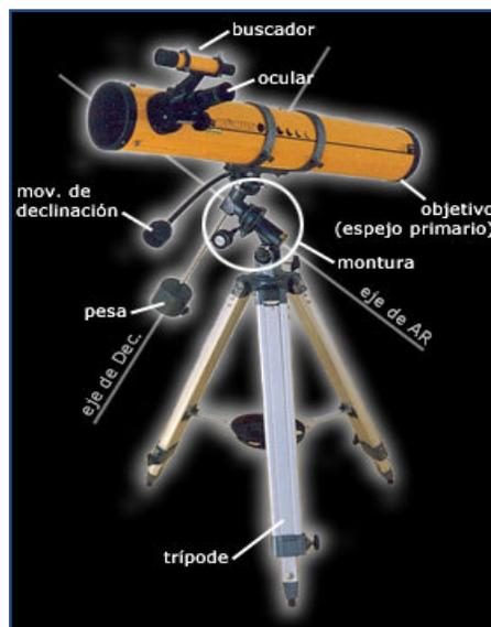
Figura 2.7 Telescopio reflector newtoniano
