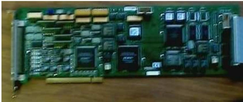
Figura A.4: Tarjeta PCI-Flex Motion-6C
