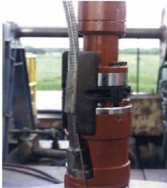
Figura 25. Conexión Mufa-Motor. (WCP Artificial Lift Systems, Schlumberger).
