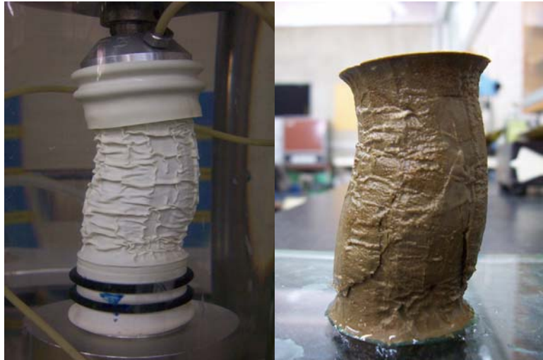
Foto 5.13. Probeta OCR = 8, 0.1 %/h
