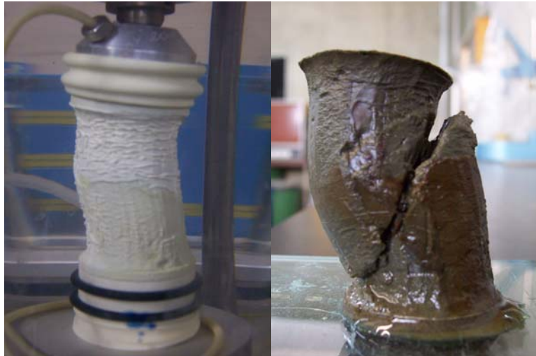
Foto 5.5. Probeta OCR = 3, 0.1 %/h
