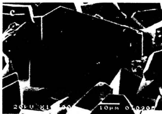
Fig 1 (a) A view of micro-crystals of EuMnGe_2O_7 , formed on the quartz tube wall. SEM-500X. (b) Crystals with morphology compatible with the disphenoidal shape in the point group 222. SEM-1000X. (c) A single crystal exhibiting the same morphology characteristic in orthorhombic symmetry. SEM-1500X.
