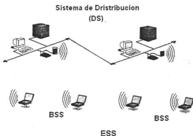
Fig. 2.11 Extended Service Set (ESS)
