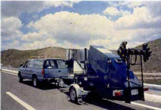
Foto 3 Falling Weight Deflectometer, KUAB
