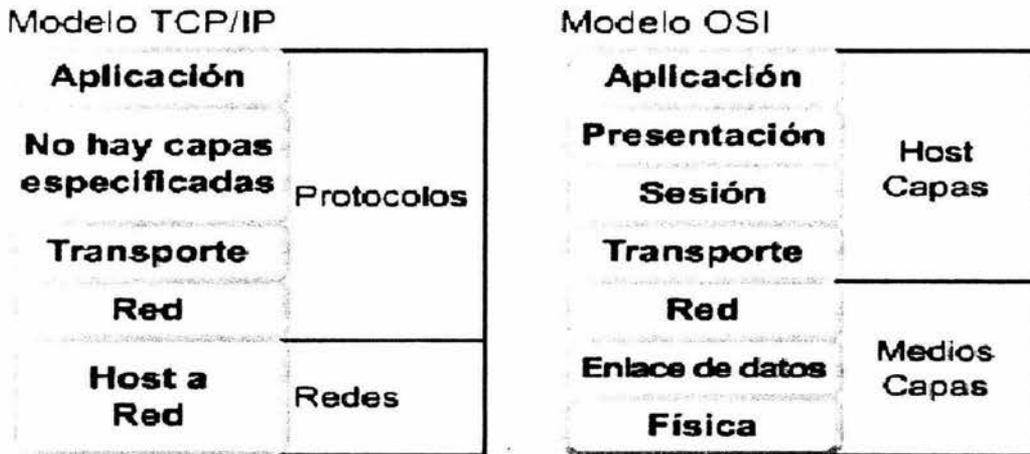
Fig. 2.1 TCP/IP vs OSI
