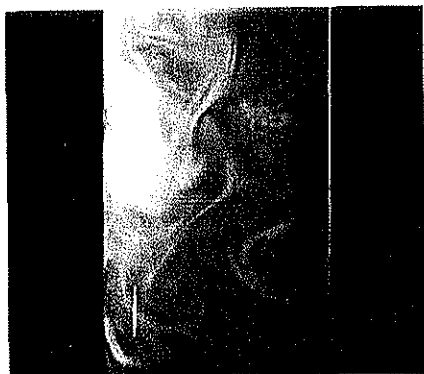
Figure 6. LIF picture showing unsteady-laminar convection. Tube diameter = 19.85 mm; Tube length = 300 mm; concentration difference = 0.025 g/cc.
