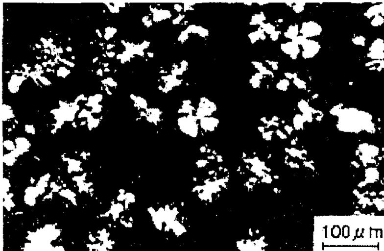
**Figura 8.** Cristales solvatados de UHMWPE (Gel-like Spherulite).<sup>9</sup>
