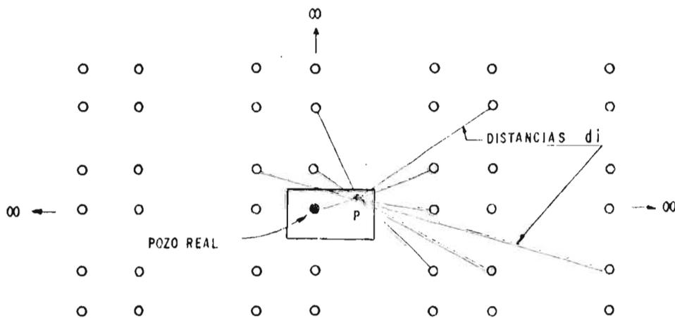
FIG. N°E-3: IMAGENES DE UN POZO EN UN YACIMIENTO RECTANGULAR CON FRONTERAS IMPERMEABLES.
