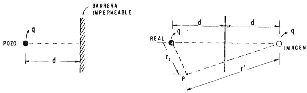
FIG. N°E-1: POZO IMAGEN EN UN YACIMIENTO CON UNA FRONTERA IMPERMEABLE.
