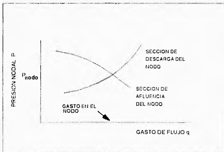
FIG. 1.2 CURVAS DE AFLUENCIA Y DESCARGA DEL NODO.
