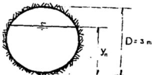
$$\begin{aligned} Q &= 2 \text{ m}^3/\text{s} \\ S &= 0.0004 \\ n &= 0.025 \end{aligned}$$
