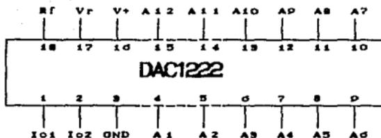
$$V_{OUT} = -V_{REF} \times C \left( \frac{A1}{2} + \frac{A2}{4} + \frac{A3}{8} + \dots + \frac{A12}{4096} \right)$$
