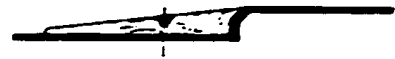
Alternative B Existing threshold remains but an addition to the threshold is constructed across the whole width
