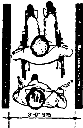
Figure 5.1.4A Minimum corridor width. Does not allow passing.
