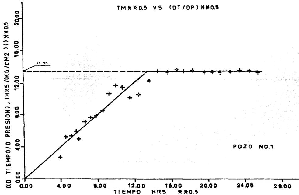
FIG. IV.1B CURVA PARA DETERMINAR EL VALOR DE  $(\Delta t_e)^{0.5}$  CORRESPONDIENTE AL POZO No. 1.
