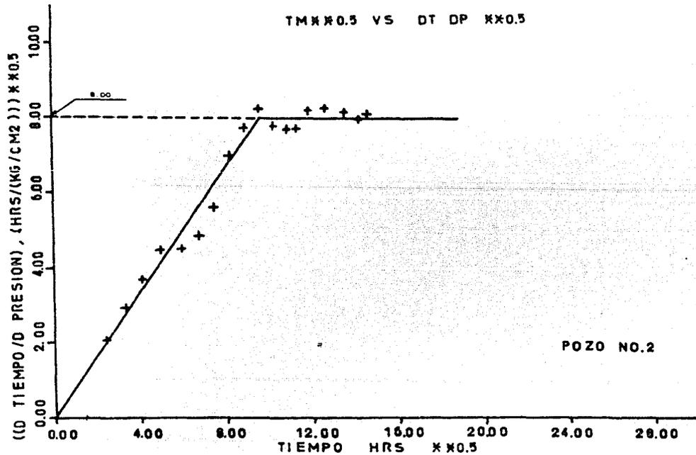
FIG. IV.2B CURVA PARA DETERMINAR EL VALOR DE  $(\Delta t_e)^{0.5}$  CORRESPONDIENTE AL POZO No.2
