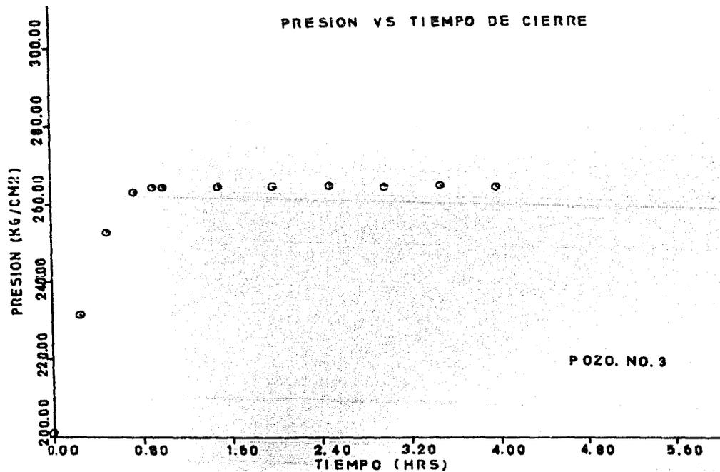
FIG. IV.3A CURVA DE INCREMENTO DE PRESION CORRESPONDIENTE AL POZO NO. 3
