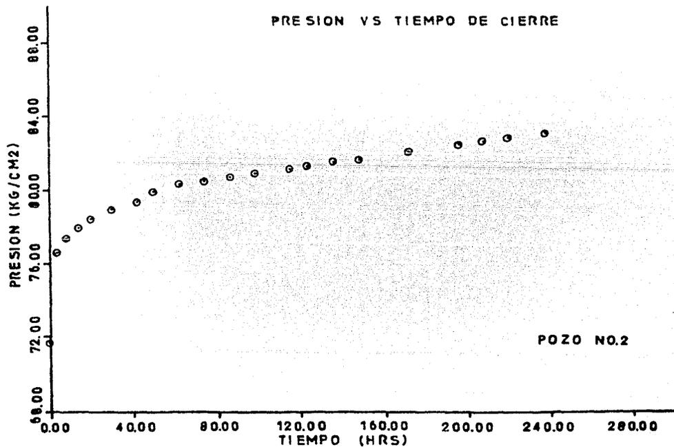
FIG. IV. 2A CURVA DE INCREMENTO DE PRESION CORRESPONDIENTE AL POZO NO.2
