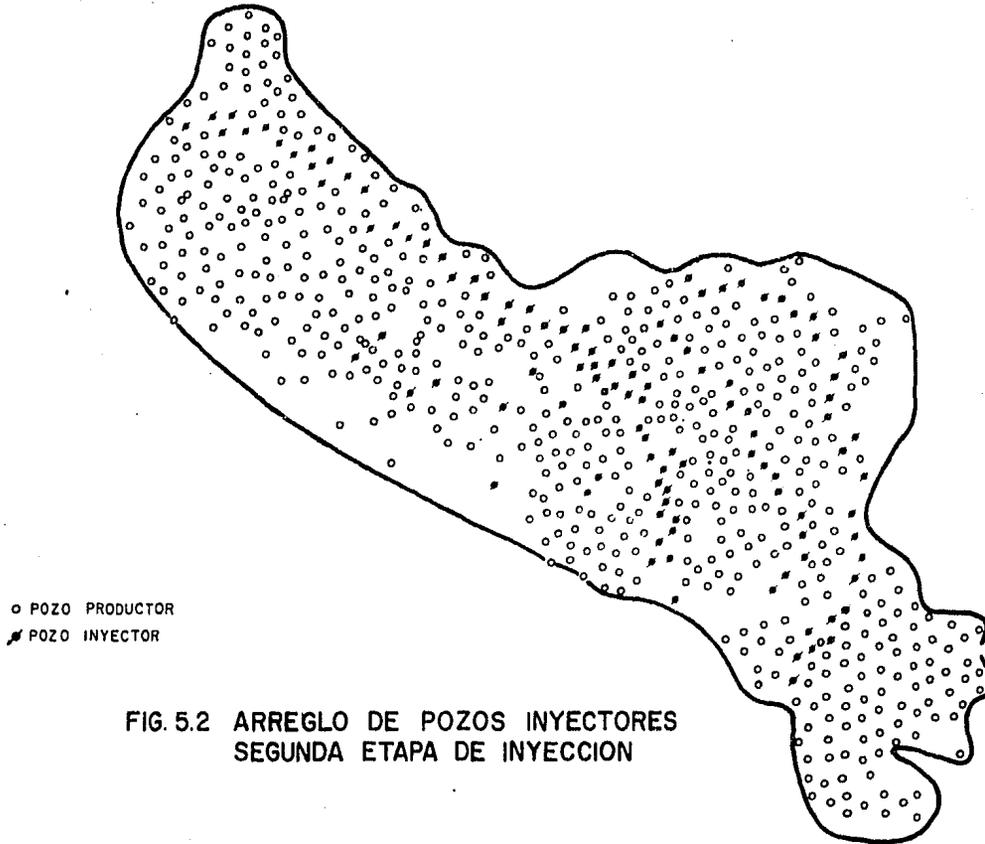
FIG. 5.2 ARREGLO DE POZOS INYECTORES
