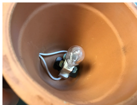
Fig. 3.5: Halogen lamp used to heat the sample.
