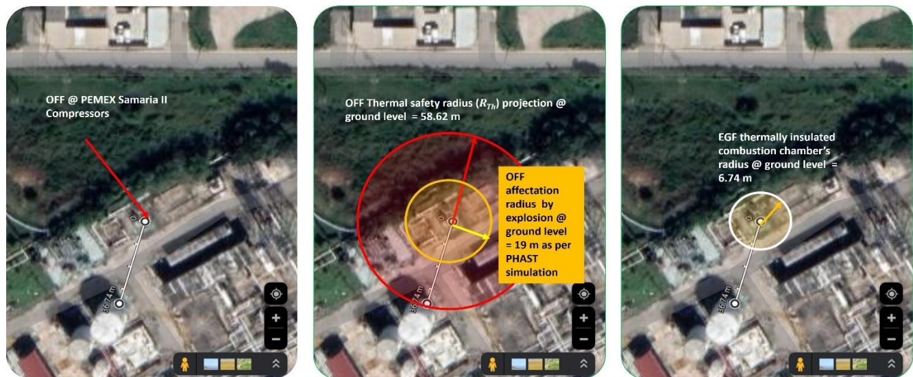
Fig. 13. On-site view with comments for the OFF and EGF case study Source: Own work
