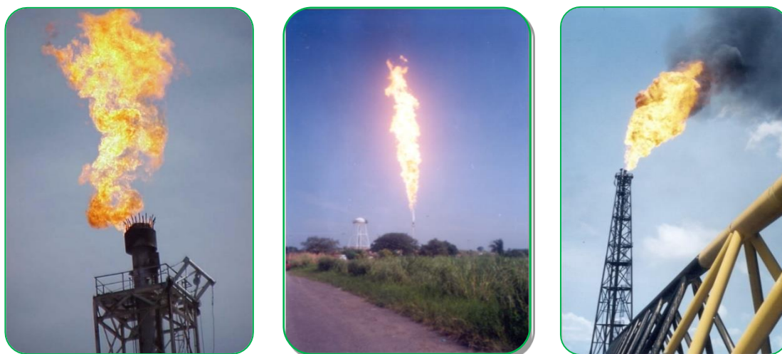
Fig. 1. Onshore & Offshore applications of Open Flame Flares (OFFs)
