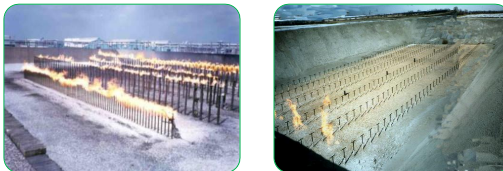
Fig. 3. Onshore applications of Open Ground Flares (OGFs)
