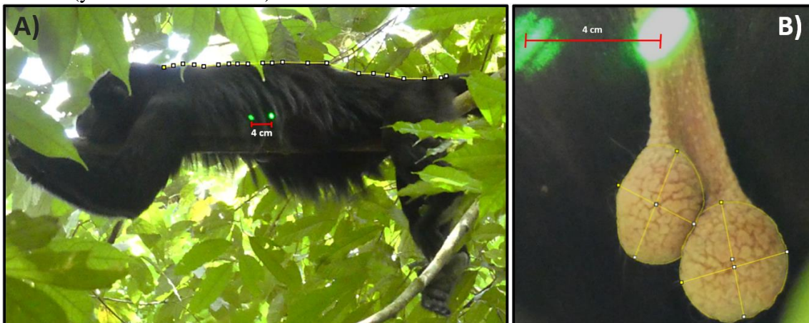
Figure S2. Parallel laser photogrammetry technique to measure non-invasively body size (A) and testicular volume (B) from 14 adult Alouatta pigra males. Green laser points positioned parallel and 4 cm apart are projected into both pictures. To measure body size, we drew a segmented line (yellow dotted line) following the contour of the male's back from the nape of his neck to the base of his tail. To measure testicular volume, we first drew an oval vector (yellow) delimiting each testicle. We then drew relatively vertical and horizontal lines, considering the inclination of the oval, to measure length and width of each testicle (yellow crossed lines).
