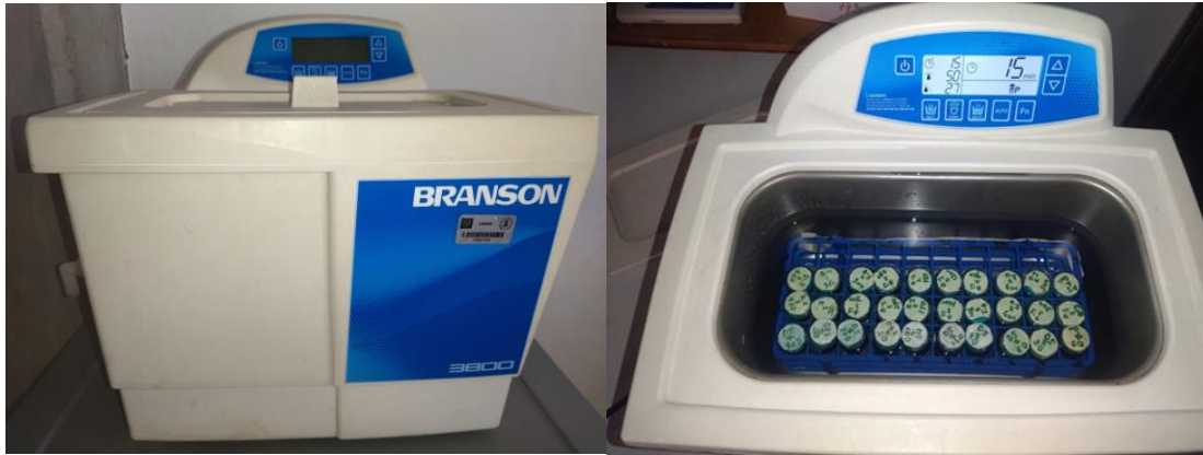
Figure 3.10 The ultrasonic bathing of the sample and the ultra-sonic machine
