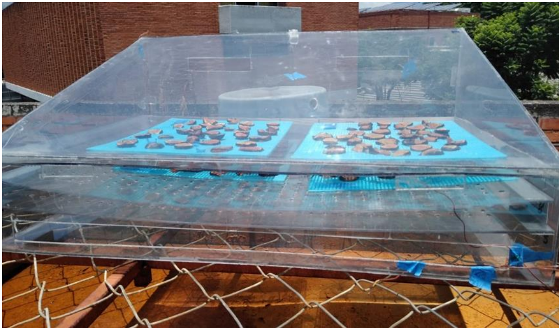
Figure 3.2 The ordinary polycarbonate bench-top cabinet dryer (ORD)
