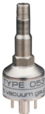
The 531 Thermocouple Gauge Tube is the time-proven, low-cost solution for continuous and accurate indication of rough vacuum pressure from  $1 \times 10^{-3}$  to 2.0 Torr ( $1 \times 10^{-3}$  mbar to 2.7 mbar). Featuring rugged dependability and consistent operation unaffected by mounting orientation.
