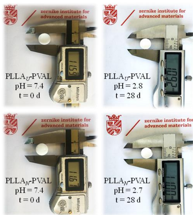
Figure 23. Profile degradation of PLLA N -PVAL and PLLA U -PVAL after 28 days at 37 °C (a) sample before and (b) after degradation test. At pH values (2.8) of final PBS solution (initial pH=7.4).
