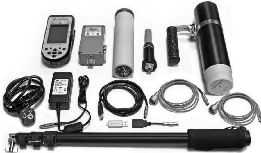
Figura 8. Detector Gaseoso de Centelleo POLIMASTER PM1403. Directindustry. Disponible en: https://www.directindustry.es/prod/polimaster/product-23674-1633890.html .
