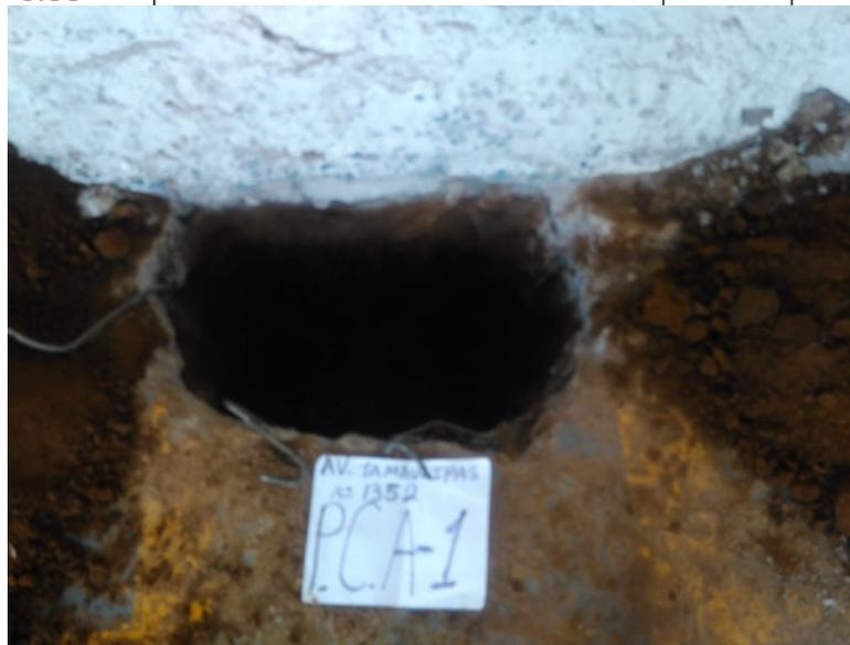
**FIGURA 11. POZO A CIELO ABIERTO (PCA-1)**
