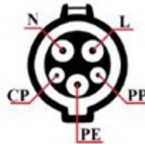
Figura 3.5: Conector SAE J1772
