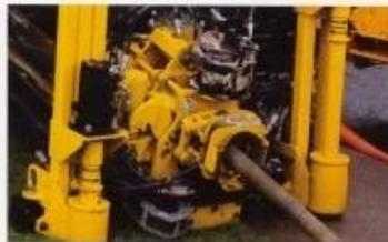
**THREE'S COMPANY.** Featuring an exclusive, patent-pending vise assembly consisting of three sets of vises coupled with a control system to optimize productivity and longevity of drill rod.
