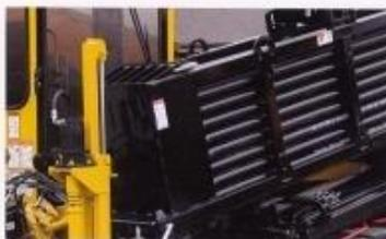
**ROD CARRYING CAPACITY.** The D36x50DR Series II carries up to 500' (152.4 m) of drill rod, reducing the need to load additional rod when performing extended bores.
