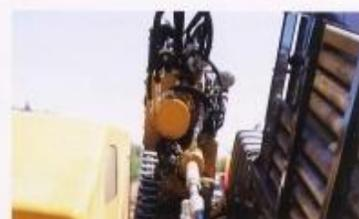
**DUAL ROD TECHNOLOGY.** Contractors can meet the challenges of their jobsite with Vermeer dual rod technology. With an industry exclusive dual threaded joint, the inner rod provides torque to the drill head, while the outer rod offers steering capability to the drill head and additional rotational torque.
