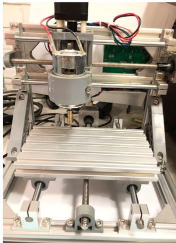
Figura 1.10: Router CNC
