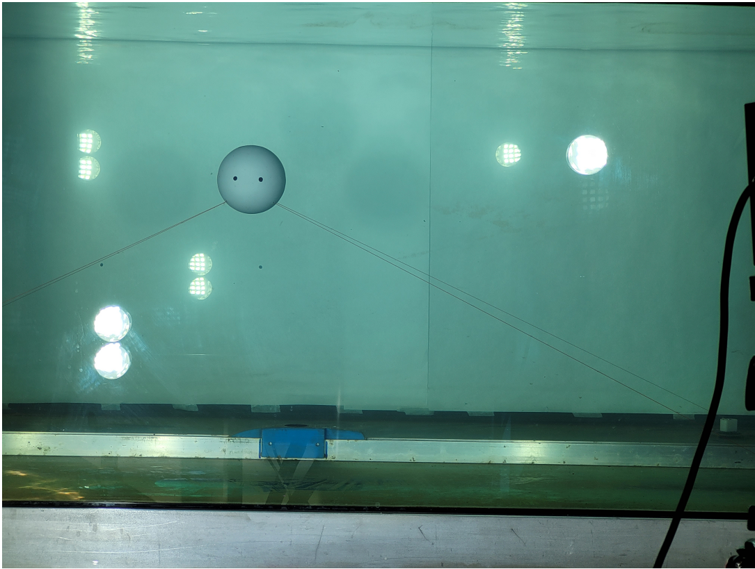
Figure 4.8: Experimental setup for series B, taken during experiments with the pumps at 35 Hz.
