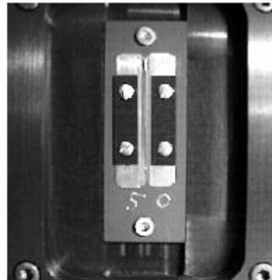
Fixed Width Slit Plate Note Orientation for Correct Installation
