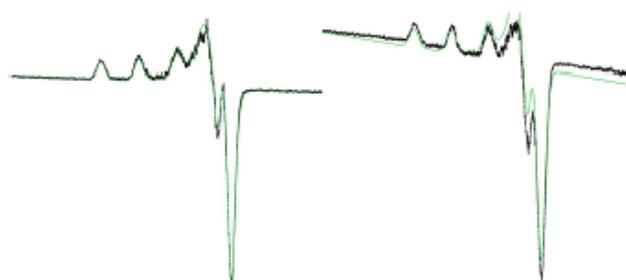
Fig. 9. (Black) Experimental and (green) simulated first derivative X-band EPR spectra of  $[\text{Cu}(\text{L1})(\text{NO}_3)]^+$  (**1a**) (left), and  $[\text{Cu}(\text{L1})(\text{dmbpy})]^+$  (**1b**) (right), prepared in DMSO solution at a 70 K. (For interpretation of the references to color in this figure legend, the reader is referred to the web version of this article.)
