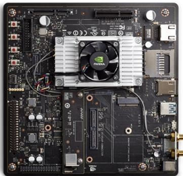
**Figura 5.3:** Jetson TX2 Developer Kit de NVIDIA.
