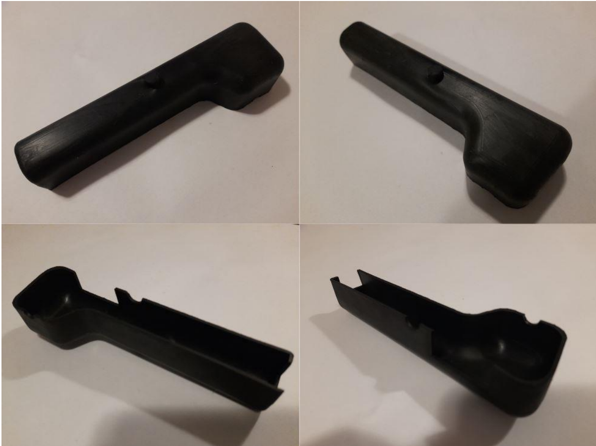
Figure 27. Photos taken to the TPE Laprene® plastic part after it was injected by the IMM
